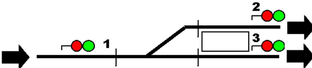
Train x is signalled from Signal 1 to Signal 2 at the end of a station platform. The train stops at the station. As the train has not cleared all the track circuits within the Route, the Route stays set. Train y is now waiting at Signal 1 and wants to go to Signal 3. This Route is clear but the original Route is still set. There must be a method for the initial Route to timeout once the train arrives at the platform so a second Route can be set.
