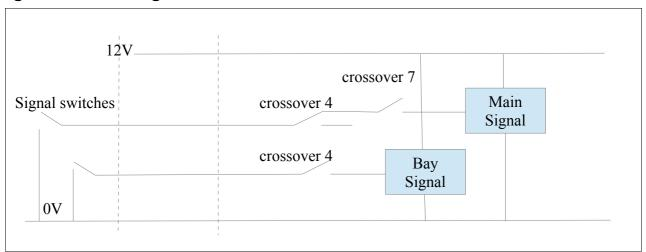
Interlocking of the main starter signal needs a relay driven by the point lever switch for crossover 4 (bay exit), and crossover 7 (goods exit). Interlocking of the bay starter signal needs another set of relay contacts on crossover 4 (bay exit). So a DPDT relay on crossover 4.
